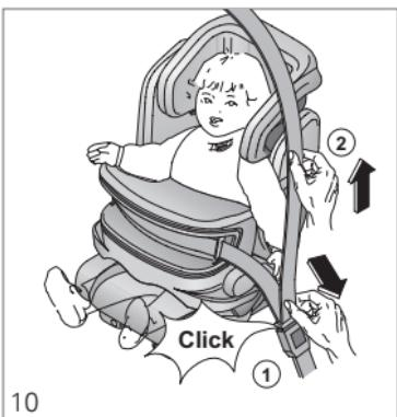
Then place the vehicle seat belt around the child car seat as shown. Once the lap belt section is in the belt guide, pull the belt tight with the shoulder section.
