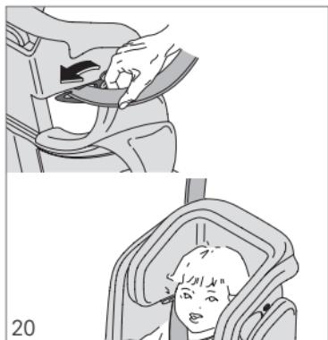
Then insert the diagonal belt into the belt guide on the head rest. The shoulder belt may only lead backwards from the child's perspective! If necessary, only use the car seat on the vehicle's back seat.
